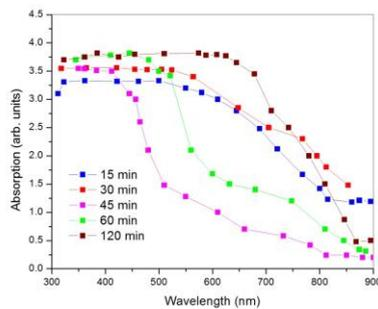
**Fig. 4 Absorption spectra of CdTe nanoparticles refluxed for different time**
