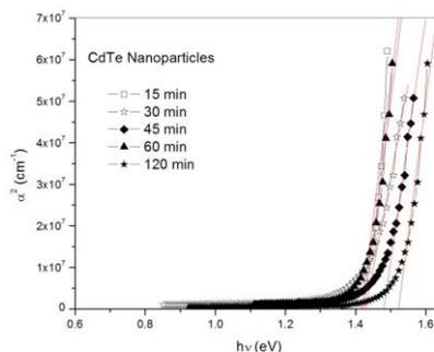
**Fig. 5 Variation in band gap energies of CdTe nanoparticles refluxed for different time**
