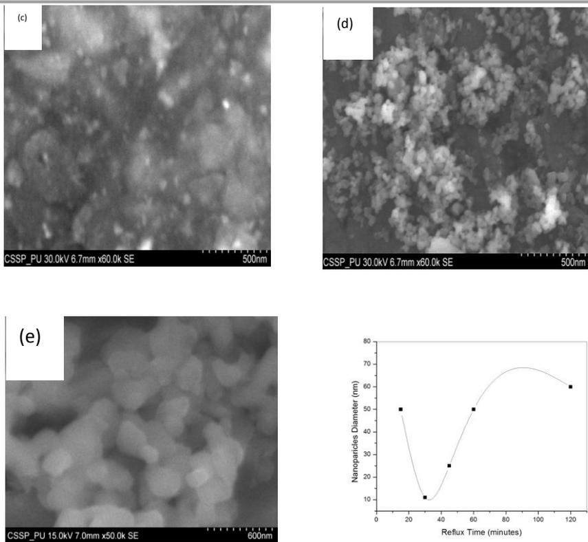
**Fig. 3** SEM micrographs of CdTe nanoparticles refluxed for (a) 15 min, (b) 30 min, (c) 45 min, (d) 60 min (e) 120 min and (f) Plot between nanoparticles' diameter and reflux time.
