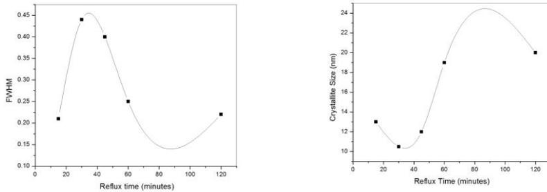
**Fig. 1 (a) FWHM and (b) crystallite size of CdTe nanoparticles at different reflux times**
