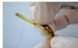
**Fig 4: Calcareous deposits inside the tube**
