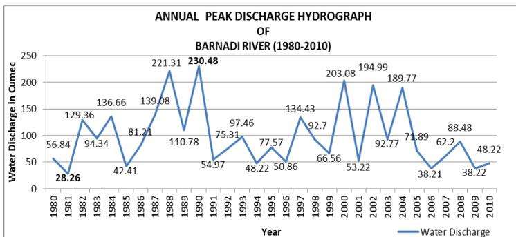
**Fig 2: Peak Discharge Hydrograph of Barnadi River (1980-2008) for N.T. road crossing site**
