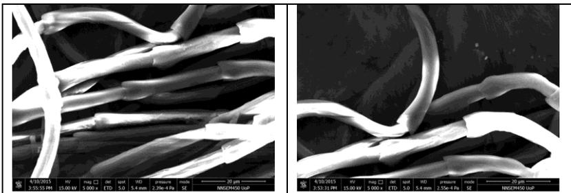
Fig 5: SEM of Control feather showing intact surface of barbules
