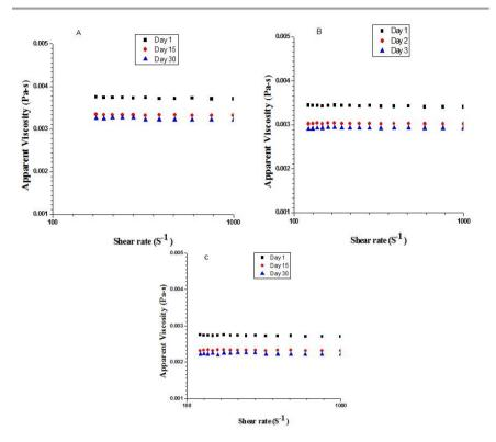
Figure: 3 Effects of storage time on the rheological properties of nanoemulsions containing variable ratios (A) 1:9, (B) 3:7 & (C) 5:5 % v/v EU:CA at room temperature.
