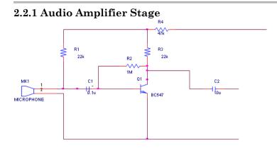
Figure 2 Audio amplifier stage
