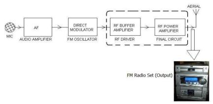
Figure 1 Block diagram of wireless FM bug showing the three stages
