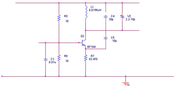
Figure 3 FM Oscillator module
