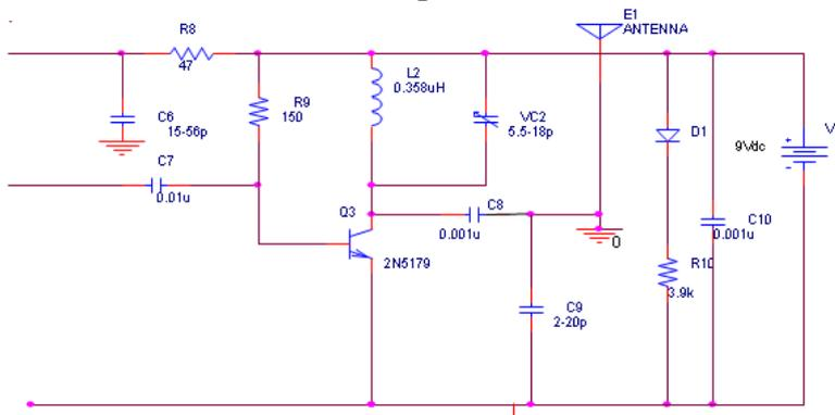
Figure 4 Schematic diagram of the RF buffer/power amplifier stage
