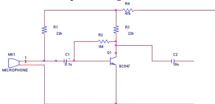
Figure 2 Audio amplifier stage
