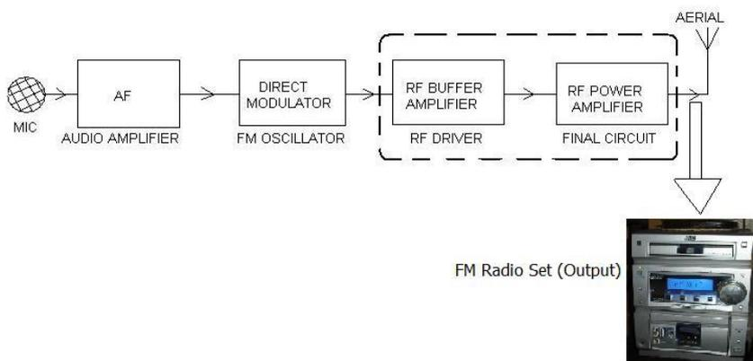
**Figure 1** Block diagram of wireless FM bug showing the three stages
