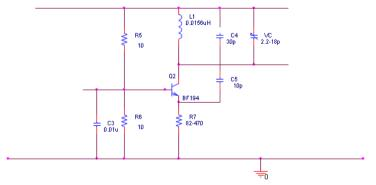
Figure 3 FM Oscillator module
