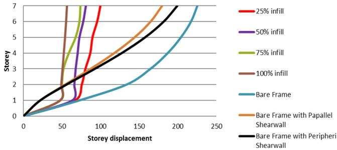
**Fig 9 : The comparison of lateral displacement between different cases having 25%infill, 50% infill, 75% infill, 100 % infill, bare frame, bare frame having parallel shear wall, bare frame with periphery shear wall**
