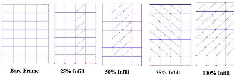
Fig 4: Elevation view for Bare Frame, 25%, 50%, 75%, 100% infill
