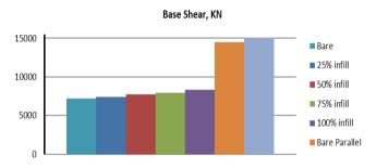
Fig 7: The comparison of Base Shear between different cases having 25% infill, 50% infill, 75 % infill, 100 % infill, bare frame, bare frame having parallel shear wall, bare frame with periphery shear wall
