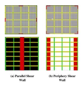
Fig 5: (a) Plan and elevation view for bare frame with Parallel shear wall (b) Plan and elevation view for bare frame with Periphery shear wall
