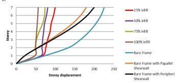
Fig 9 : The comparison of lateral displacement between different cases having 25% infill, 50% infill, 75% infill, 100 % infill, bare frame, bare frame having parallel shear wall, bare frame with periphery shear wall
