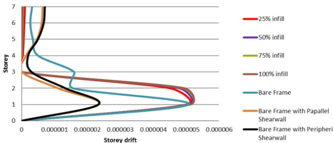
**Fig 11: The comparison of story drift ratio different cases having 25%infill, 50% infill, 75 % infill, 100 % infill, bare frame, bare frame having parallel shear wall, bare frame with periphery shear wall**
