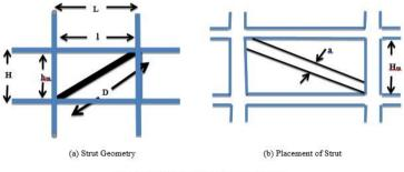
Fig 3: (a) Strut Geometry (b) Placement of Strut Credit: R. Shahrin & T.R. Hossain (2011)
