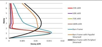
Fig 10 : The comparison of story drift between different cases having 25% infill, 50% infill, 75 % infill, 100 % infill, bare frame, bare frame having parallel shear wall, bare frame with periphery shear wall
