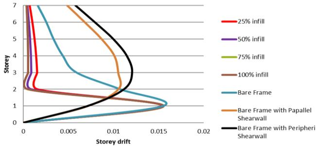
**Fig 10 : The comparison of story drift between different cases having 25%infill, 50% infill, 75 % infill, 100 % infill, bare frame, bare frame having parallel shear wall, bare frame with periphery shear wall**
