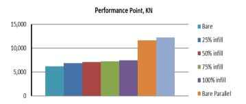
Fig 6: The comparison of performance point between different cases having 25% infill, 50% infill, 75% infill, 100% infill, bare frame, bare frame having parallel shear wall, bare frame with periphery shear wall
