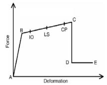
Fig 1: Force-Deformation for pushover analysis
