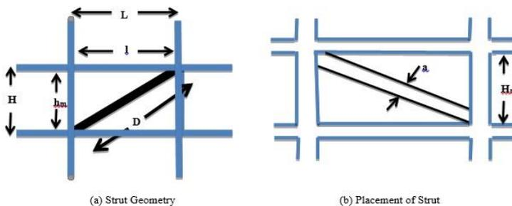
Fig 3: (a) Strut Geometry (b) Placement of Strut
