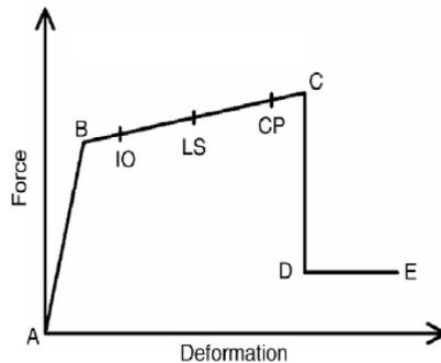
**Fig 1: Force-Deformation for pushover analysis**
