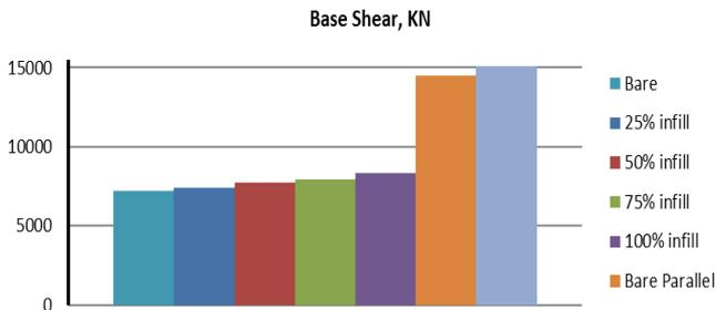
**Fig 7: The comparison of Base Shear between different cases having 25%infill, 50% infill, 75 % infill, 100 % infill, bare frame, bare frame having parallel shear wall, bare frame with periphery shear wall**
