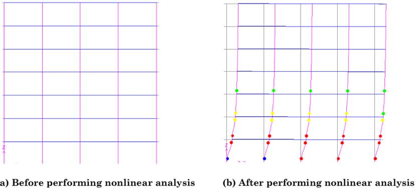
**Fig 8: Formation of plastic hinge in bare frame after performing nonlinear analysis**
