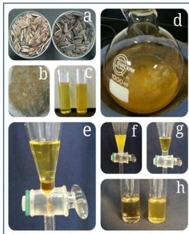
**Fig. (1): Transesterification of Sunflower (*Helianthus annuus*) oil by CaO as catalysts.**(a) Shahrazour (left) and Bazian (right) seeds.(b) Powder of seeds. (c) Crude oil (right) and Refin oil (left). (d) Mixing of oil, methanol and CaO. (e) Separation of biodiesel. (f) Washing of biodiesel. (g) Separation of biodiesel after washing. (h) Refine biodiesel of Shahrazour (left) and Bazian (right) .
