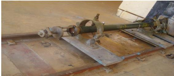
**Figure 20: Ground static Test Setting(SRM on the static test stand)**
