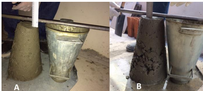
Figura 2 – (A) Slump teste T1, (B) Slump teste T2.
