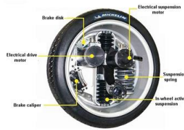
Figure 2: Michelin active wheel with in-wheel motor.
