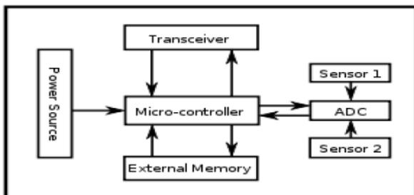
Figure 1: Structural view of WSNs
