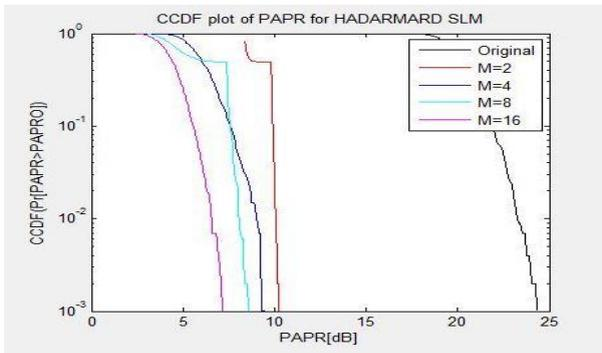
**Fig.2: CCDF plot of PAPR for HADARMARD\_SLM**
