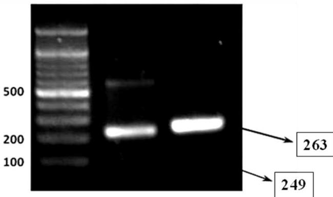
**Figure 3:** Ethidium bromide staining of amplified DNA fragment size separated on a 1% (wt/vol) agarose gel. PCR products of a 214bp bFGF fragment amplified by Forward Primer and Reverse Primer. The actual size of fragment is 15bp longer because of the linker sequence of Reverse Primer. GC-clamped PCR products of the *bFGF* fragments generated by two consecutive amplifications. The size marker is a 100-bp DNA ladder (FERMENTAS).
