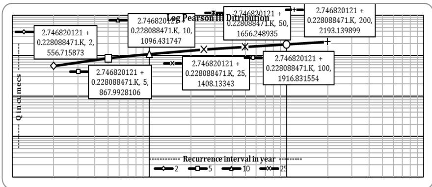
**Fig. 6: Flood frequency analysis of the Puthimari River by log Pearson III method for recurrence interval of 2, 5, 10, 25, 50, 100 and 200 years**
