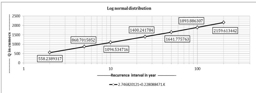
**Fig. 5: Flood frequency analysis of the Puthimari River by Log-normal method for recurrence interval of 2, 5, 10, 25, 50, 100 and 200 years**
