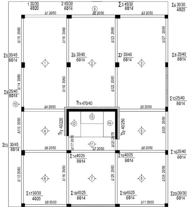
Figure 7: Formwork of strengthened structural system for performance case "b".
