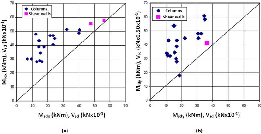
Figure 6: Correlation diagrams (a) for x-x direction, (b) for y-y direction for the strengthened building of case "a".
