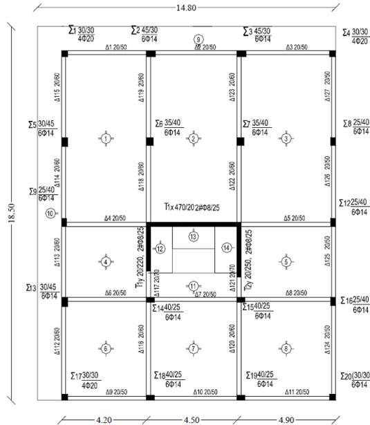
**Figure 2: Formwork of ground floor slab of the existing building.**
