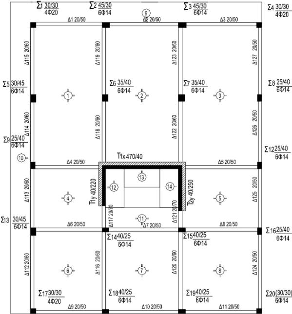
Figure 5: Formwork of strengthened structural system for performance case "a".
