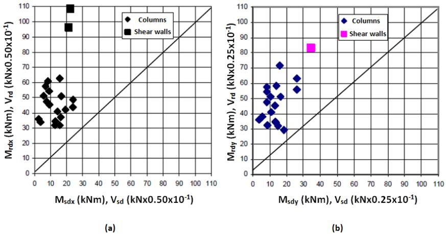
Figure 8: Correlation diagrams: (a) for x-x direction, (b) for y-y direction for the strengthened building of case "b".
