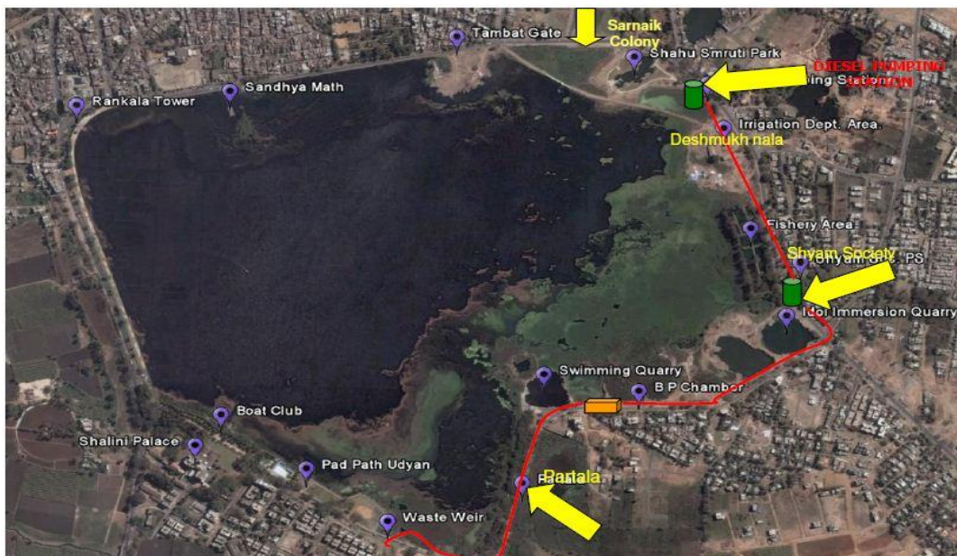
Fig 3: Sources of sewage to Rankala Lake and Water sampling points in Rankala
