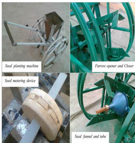
Fig. 2: Photo graph of component parts of the fabricated maize planter
