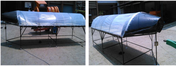
Fig.1 Photographics view of solar tunnel dryer
