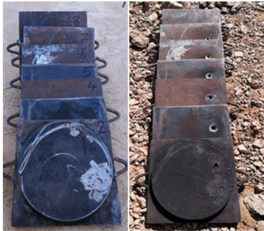
Figure 11: Steel plates before and after penetration test
