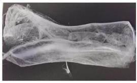
Figure 1 – Synthesized PLLA membrane obtained from rotary jet spinning process [2].
