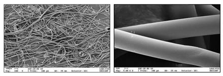
Figure 2 – Scanning electron micrographs of PLLA membranes at magnifications of 100x and 5000x.
