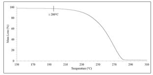
Figure 4 - PLLA membrane thermogravimetric curve.
