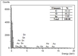
Figure 3 - Spectrum by EDS analysis [2].
