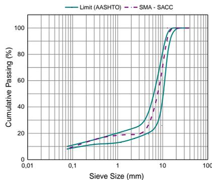
**Figure 1. Granulometric curve of the composition with SACC, according to the maximum nominal size**
