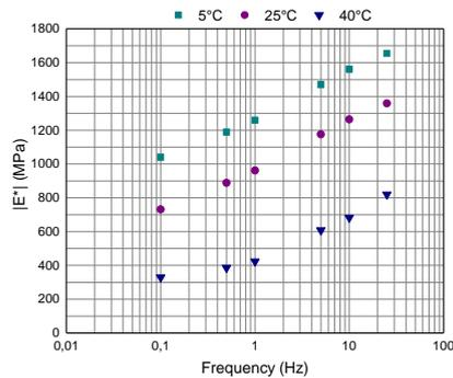
**Figure 4. Dynamic modulus x frequency, SMA-SACC**
