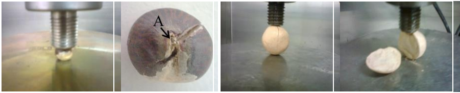
Figure 06. Visual Aspect of the Açai Seed (A And B) and SCCA Grains (C And D) after performing the Simple Compression (SC) Tests
