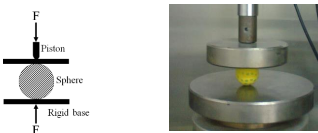
Figure 02. Scheme of the SCCA Grains and Açai Seeds subjected to the Simple Compression Test
