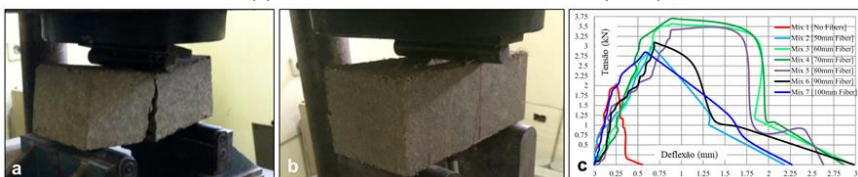
Figure 1. Ceramic block not reinforced (a) and reinforced with fiber (b) under the same tension; Graph Tension x Deflection of the block reinforced with fibers in different mm (c). Source: Mostafa and Uddim (2016).
