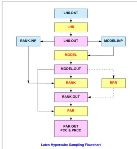
**Figure 1 Flow diagram of LHS techniques**
