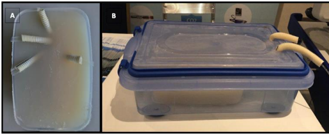
Figure 2. A) Dacron prosthesis in an agar tissue-mimicking material. B) Plastic box with water and openings for exteriorization of the iliac branches.
