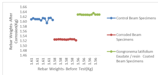
Figure 3.7: Rebar Weights- Before Test versus Rebar Weights- After Corrosion (Non-Corroded, Corroded and Resin Coated Specimens)
