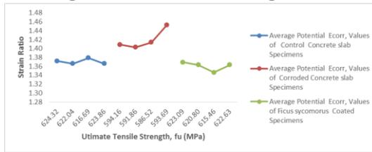
**Figure 3.3B: Average percentile Ultimate Tensile Strength versus Strain Ratio**
