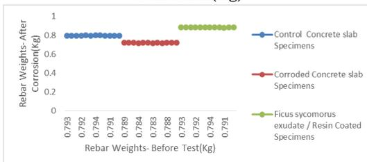
**Figure 3.6A: Average Rebar Weights- Before Test(Kg) versus Rebar Weights- After Corrosion(Kg)**
