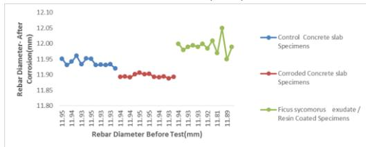
**Figure 3.4A: Average Rebar Diameter Before Test(mm) versus Rebar Diameter-After Corrosion(mm)**
