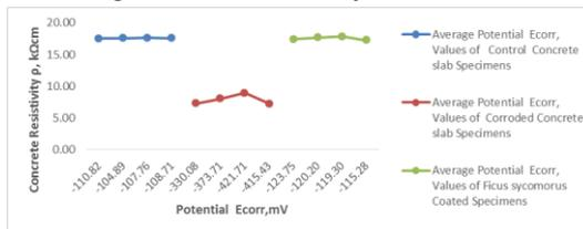
**Figure 3.1B : Average Percentile Concrete Resistivity versus Potential Relationship**
