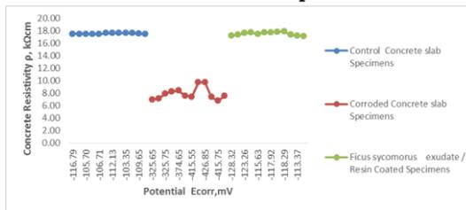
**Figure 3.1A: Average Concrete Resistivity versus Potential Relationship**
