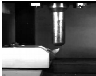
Figure 3. Frame of the film obtained by the high-speed camera at the MIBE, with the specimen positioned according to Soares et al., 2005.
