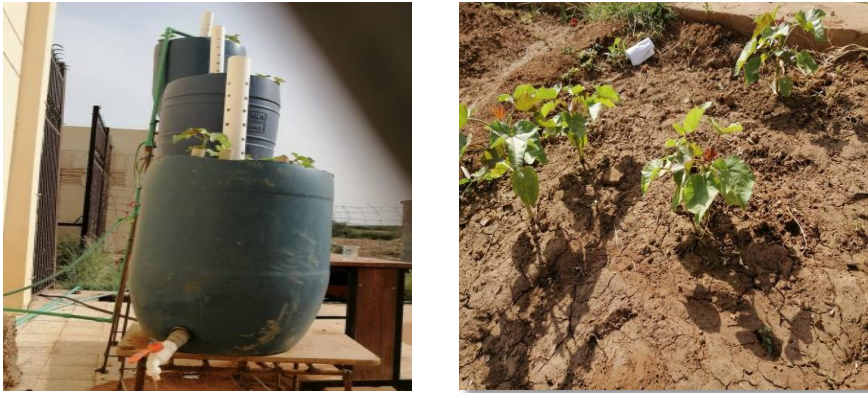
Fig.3. Constructed wetland planted with Jatropha
