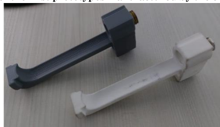
Figure 7. Images of the first prototypes manufactured by the 3D printing method
