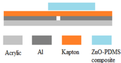
Figure 1: Schematic of fabricated PDMS-ZnO composite FD-TENG
