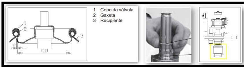
Figure 5 - on the left is the valve crimped onto the can; in the center is the clamp being assembled; on the right is the crimping head.
