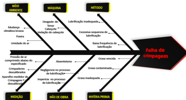
Figure 6. Failure Cause Analysis
