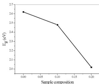
**Fig.5.** Variation of band gap with composition of barium titanate/PANI nanocomposites
