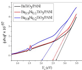
**Fig. 4** Band gap of barium titanate/PANI nanocomposites
