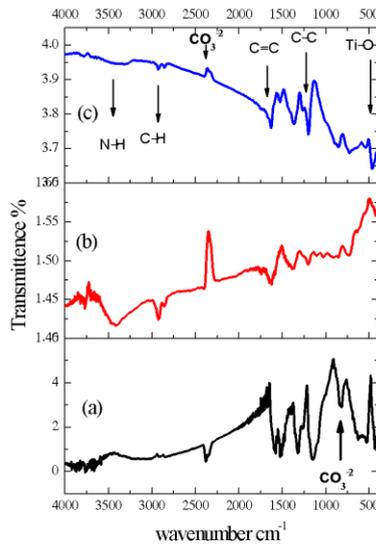
**Fig.2** FTIR spectra of barium titanate/polyaniline nanocomposites (a) BaTiO<sub>3</sub>/polyaniline, (b) Ba<sub>0.9</sub>Ni<sub>0.1</sub>TiO<sub>3</sub>/polyaniline, and (c) Ba<sub>0.8</sub>Ni<sub>0.2</sub>TiO<sub>3</sub>/polyaniline
