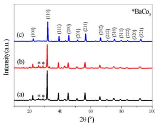
**Fig. 1.** XRD spectra for barium titanate/polyaniline composites. (a) BaTiO<sub>3</sub>/polyaniline, (b) Ba<sub>0.9</sub>Ni<sub>0.1</sub>TiO<sub>3</sub>/polyaniline, and (c) Ba<sub>0.8</sub>Ni<sub>0.2</sub>TiO<sub>3</sub>/polyaniline
