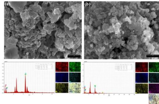
**Fig. 3** FESEM, EDX spectra and elemental mapping of barium titanate/PANI nanocomposites (a) BaTiO<sub>3</sub>/polyaniline and (b) Ba<sub>0.9</sub>Ni<sub>0.1</sub>TiO<sub>3</sub>/polyaniline
