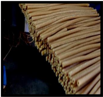
Fig. 3. Cut strand single base propellant with temporary cutting tool
