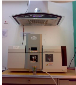
Figure1 showed samples after digestion Figure2 showed (A.A -6300-DAIGEN, SHIMAZU-JAPAN)
